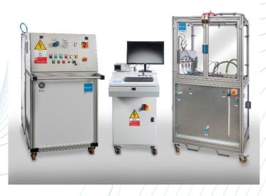
The B 23201 test bench is designed for the characterization of valves or other fluid dynamic components used in aerospace industry, using a water/glycol mixture as a fluid.
