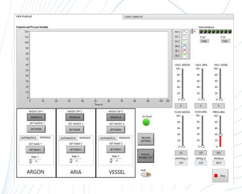
Figure, on the right, shows the control and supervision interface of 3 PID regulation loops, integrated in the HMI, but carried out by remote hardware based on an application developed ad-hoc and installed on the FPGA.
