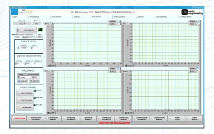
Figures, on the right, show an interface for displaying and configuring vibration measurements (in time and frequency) integrated into the HMI but carried out by dedicated hardware transparently to the operator.
