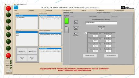
DAS allows you to control the individual devices, the operating modes (manual / automatic) and to view status and measures from the sensors in a simple and intuitive way. The system allows to insert test recipes, store recipes and execute automatic tests.
