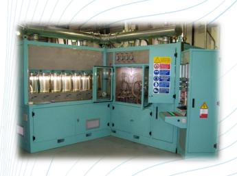
Bench designed for testing delivery and recovery pumps or combined engine oil circuit.
