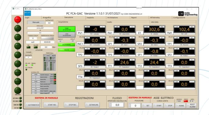
The test stand is equipped with a PC and NI data acquisition system. PC software can set the test profile and can create a complete test report.
