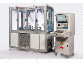
B\_23034 bench tests the Fuel Supply Units (GAC) for Diesel and Gasoline engines.
