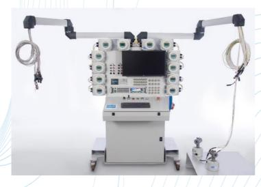
B\_23092 station is built for the measurement of the hydraulic parameters of powertrain cooling system of thermal, hybrid and/or electric vehicles.
