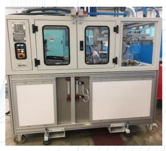
B\_222861 cart is equipped for testing the RACER pump.
