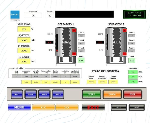
The test stand is equipped with a PC and NI data acquisition system PC software can sets the test profile and can create a complete test report [pressure vs time].
