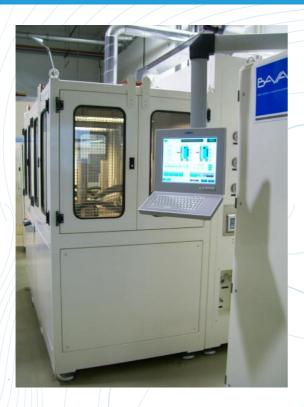
B\_22143 test bench is designed to test resistence and performances of cars heat exchangers internal ducts. It flushes on internal ducts a mixed flow of corrosive water and refrigerant fluid.
