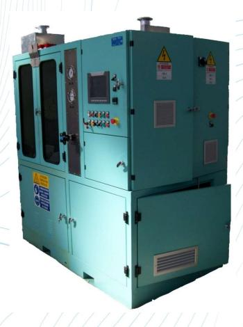
Bench designed for testing lubrication nozzles.
