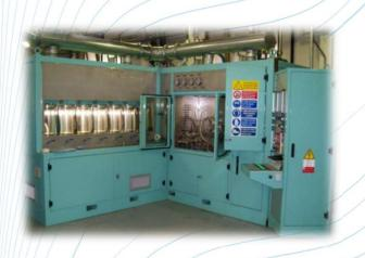
Bench designed for testing delivery and recovery pumps or combined engine oil circuit.
