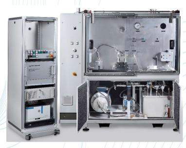
B\_23111 test bench is designed to complete functional test and force vs time diagram on servo actuated jacks for flight surfaces:
